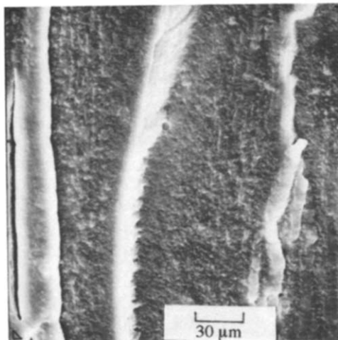
Fig. 5. Fractured surface of TPU/ABS 50/50 blend after 2 h of etching with MEK and dried at 40 °C under vacuum.
